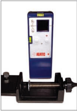
LS30 Laser Detector Hand Held or Rod Mounted lets you use the CPL50 outdoors, in very bright light conditions, or at greater distances.
